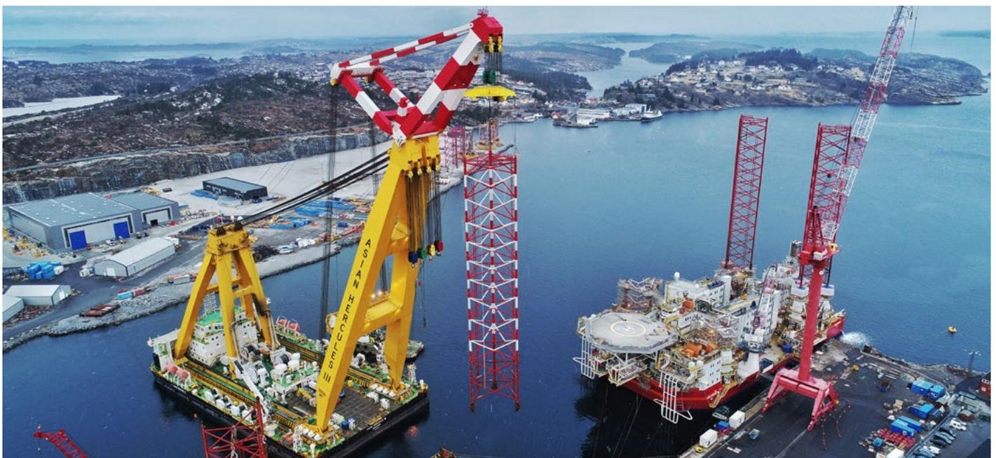
Heavy lift vessel “Asian Hercules III” installs a new leg onto the “Haven”, which has recently undergone a major upgrade
