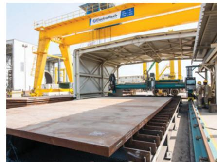
LONG SEAM CNC PLATE CUTTING, BEVELING AND CHAMFERING
