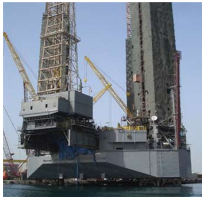
Arch Rowan leg inspection and re-furbishment.
