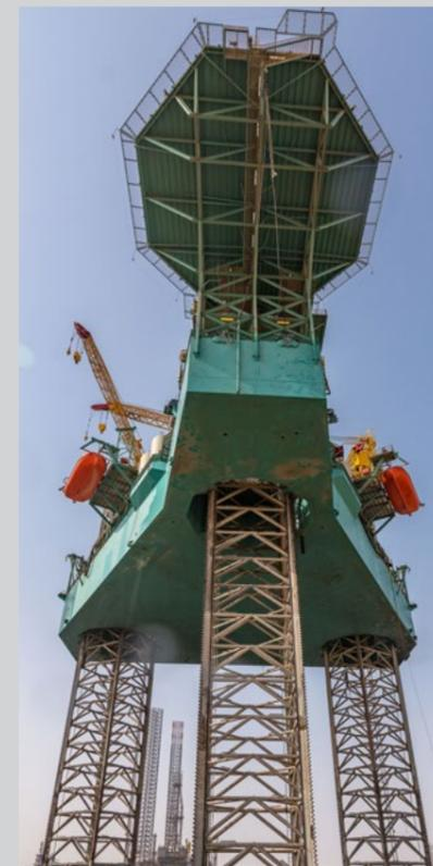
ADNOC drilling rig 'Makasib' is one of three jackup rigs Lamprell delivered within a two-week period in Q3 following refurbishment work
